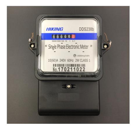
The meter is designed to measure single phase two wire AC active energy. It adopt LSI and SMT technology, the key component are long life international brand product. All of its functions comply with the relative technical requirement for class 1 single phase watt hour meter in IEC62053-21. It is a long life meter with the advantage of high stability, high over load capability, low power loss and compact size.
